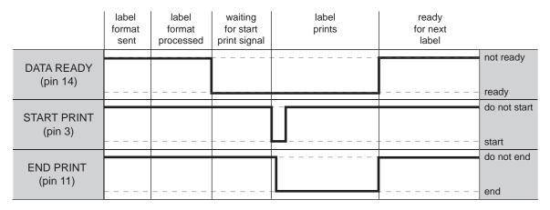
Figure 48 • Applicator Signals (Mode 2)
